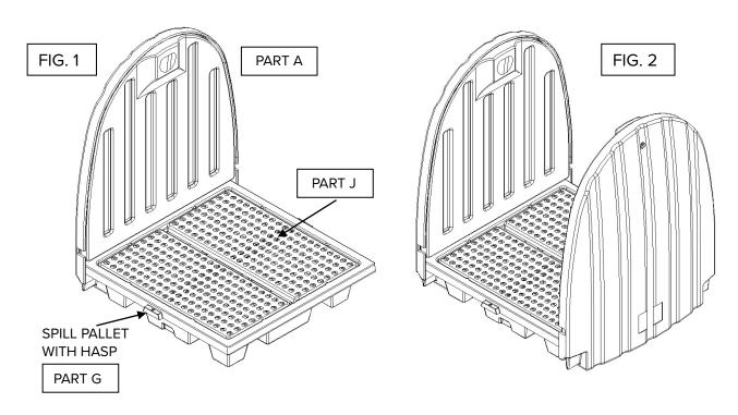
2) Place the second hardcover sidewall on the opposite side of the spill pallet. (See fig.2)
