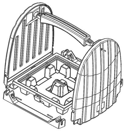
1) Stand part (A), hardcover sidewall, upwards and slide it against the edge of the spill pallet, part (G), making sure that the sides with molded in hasps are facing outward (See fig. 1). At this time place the grates, parts (J), onto the spill pallet also.
